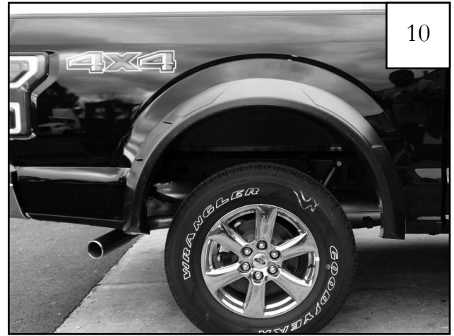
Completed rear flare installation.
